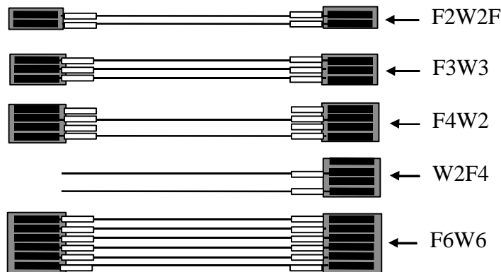
Figure 5 Illustration of several cable types.
