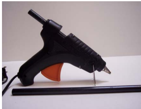
Figure 3. Hot-glue gun enables you to encapsulate cable connector solder joints to increase mechanical strength of the connection. The black cylinder of low-melting-temperature plastic glue matches the black ABS body of the robot and may be used to secure light sensors and other elements to the robot body.
