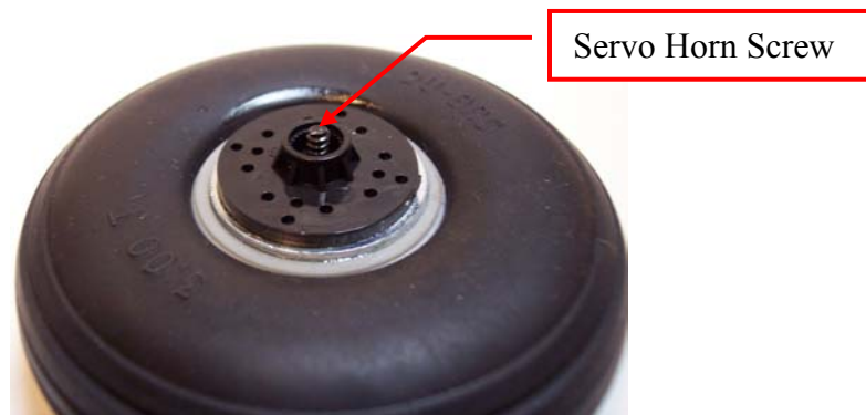
Figure 37. A Servo Horn and a 1 inch steel washer superglues to the wheel hub to allow mounting on a wheel servo.
