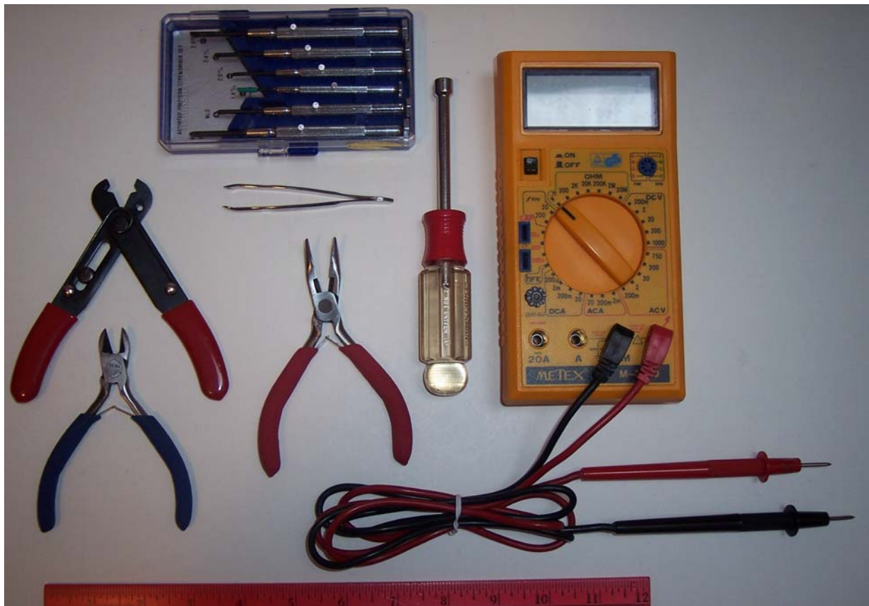
Figure 1. You will find these tools useful for assembling your Mekatronix robots. The jeweler's screwdriver set provides precision flat blade and Phillips head screwdrivers required for mechanical assembly of the robot. The tweezers allow you to easily manipulate small parts (washers, nuts, screws) while the needle nose pliers permit you to exert greater gripping forces while manipulating parts. The nut driver easily tightens 4/40 screws...but be careful not to over tighten nuts if you use this tool. The diagonal cutters and wire strippers cut wire. The wire stripper also allows you to strip wire for tinning and soldering. The multimeter is optional, but if you build electronic circuits you may want one on hand.
