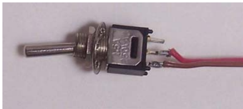
Figure 58. The red wire of the power-on toggle switch solders to the center post and the brown to one of the edge posts, which edge post does not matter.
