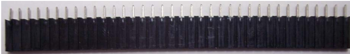
Figure 6. This enlarged view of a 36-pin female socket shows the segmentation that allows you to cut various length sockets for cable construction. In constructing cables you will tin the socket pins and then solder tinned cable wires to the pins.
