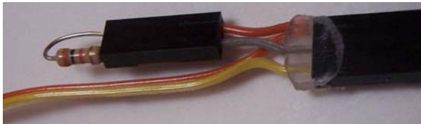
Figure 55. Details of the Photoresistor connector show the wire colors and terminations. The nominal 30K Ohm voltage divider resistor inserts into the 2-Pin Female connector, which connects to the 3-Pin Female connector. The orange wire connects to an outside pin of the 3-Pin connector and is common to the orange
