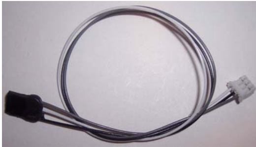
Figure 61. The three wire IR range detector cable (CIRxx) with a standard 3-Pin Female connector at one end and a locking, miniature 2mm-pin-spacing connector.
