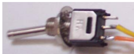
Figure 59. The yellow wire of the download/run (mode) toggle switch solders to the center post and the orange to one of the edge posts, which edge post does not matter.
