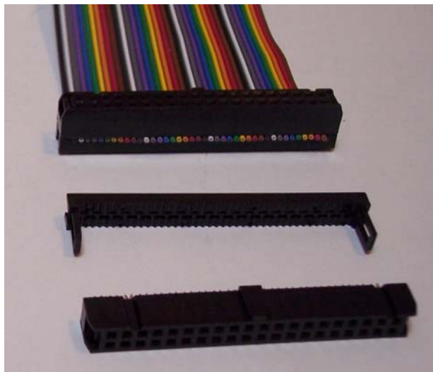
Figure 42. Forty-wire Insulation Displacement Connector (IDC) for the front bumper (10 wires), rear bumper (10 wires), and the FM bus (16 wires) mounts onto the headers at the bottom of the MEKA VR128 board. Since the headers only use 36 wires, you can strip away four end wires.
