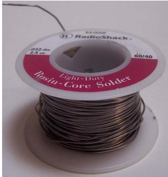
Figure 4. Depending upon your robot kit type, you may require superglue for joining robot body parts, rosin-core solder to mechanically and electrically connect cable wires to end-connectors and solder electronic components to a printed circuit board, and black-plastic glue rods for the glue gun to encapsulate soldered, cable connections for added mechanical strength or to secure sensors and other body parts.
