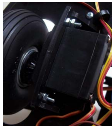
Figure 84. The left photograph shows the right and left wheel motor sockets plugged into the lower two servo/motor headers: PC1(1,2,3) and PC0(1,2,3). A wheel motor is shown mounted in the right photograph.
