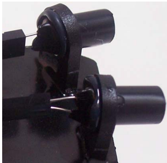
Figure 33. This picture shows the insertion of the photoresistors into the Photoresistor Holders of the Sensor Head . The shrink-wrap tubing encapsulates the wires and the back of the sensor to block out light. Black hot glue secures the sensors firmly into the holders.
