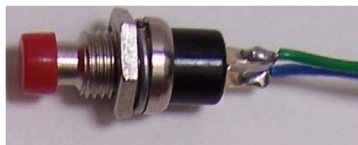
Figure 60. Solder the green wire to one terminal and the blue wire to another terminal on the reset button switch.
